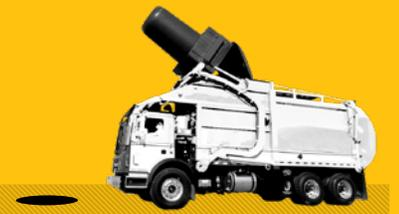
Gravity latch ensures control of mess during collection.
