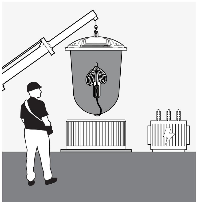
2.2.3 The bag is prepared to empty by removing the rope from the storage pocket or fabric strap.
