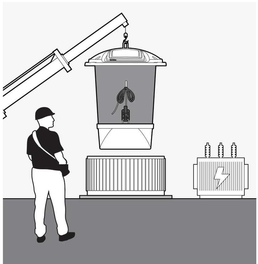
1.2.3 The bag is prepared to empty by removing the safety pin from the clamp as shown in image below. (Semi-rigid and rigid bags only).
